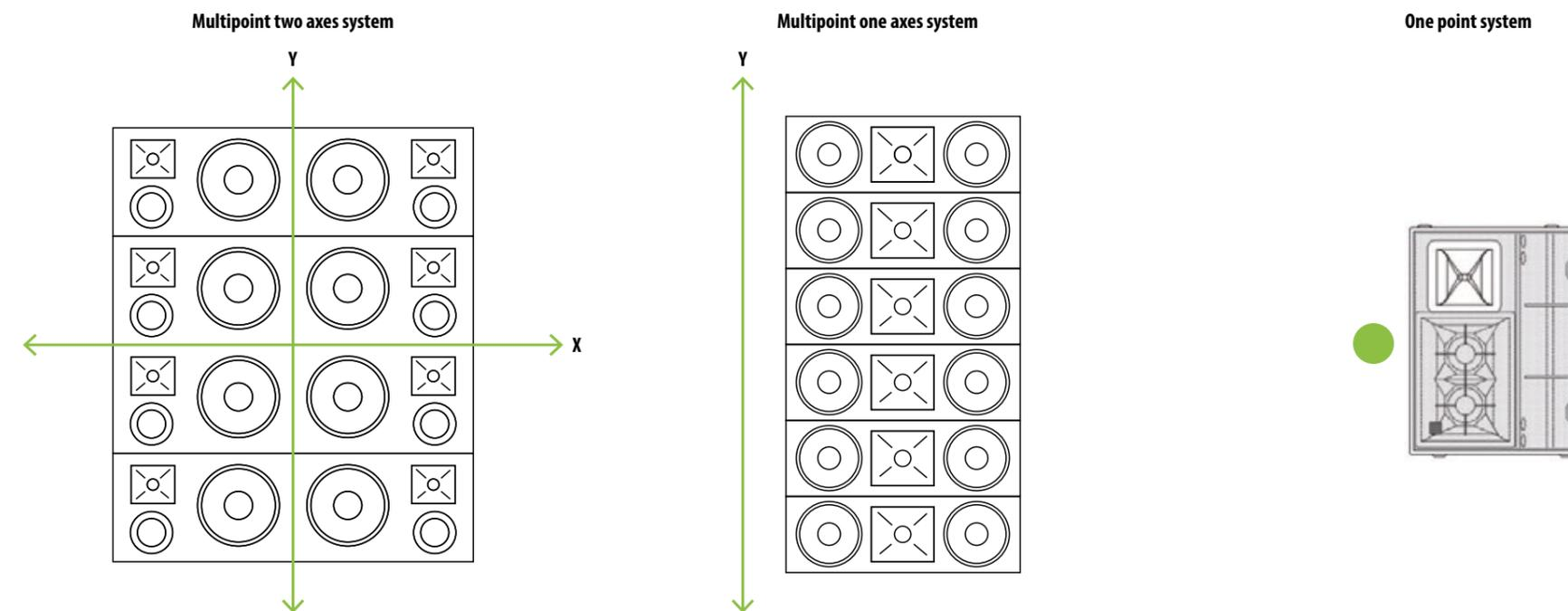
The first types of multipoint sources were simply a large pile of cabinets, stacked together like building blocks and intended to array on all axis. A major improvement in the next generation of systems was the introduction of multipoint, one-axis systems that provided better frequency response and increased definition than previous multi axes systems. Unfortunately, whilst a step forward, the frequency response and impulse responses were still not ideal and the coverage was often inconsistent.
