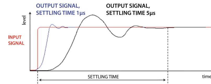
Figure B: Pulse response of an audio signal after transfer through various analog and digital systems.
