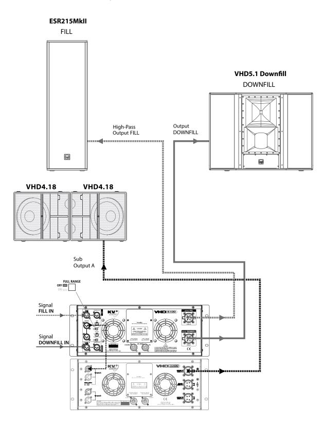
Set VHD5100 Amplifier to FULL RANGE OFF mode. Signal is crossed over at Hi/Mid for ESR215Mkll cabinets and SUB for external subwoofer. Crossover frequency is app. 70Hz.
