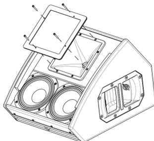
Place the protective cover over the driver horn.
