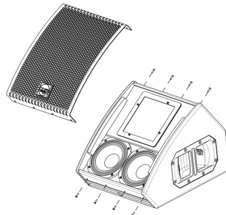
Place the grill and tighten the screws
