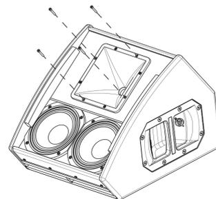
Remove 4pcs hexagon screws, size 2.5 from positions as shown.
