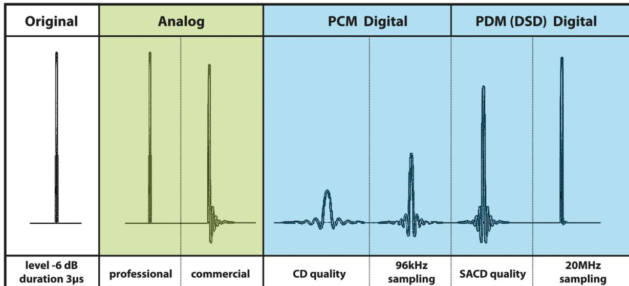
*Impulse time response audio systems to input pulse, level -6dB, duration 3μs*
