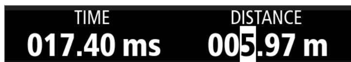
Pic 27: Rotate encoder to set value. This will change the value in 0.05ms steps which is approximately 0.02m. For that reason, when setting meters, it adds or subtracts approximately 0.02, 0.1, 1, 10, or 100 meters depending on the selected range.
