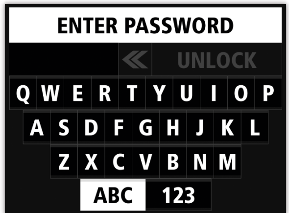
Pic 59: When amplifier is locked with password, after turning on display or turning on display or turning on from standby you need to enter this password.
