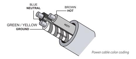
CAUTION: THE ESP2000 REQUIRES A GROUND CONNECTION. ALWAYS USE A GROUNDED OUTLET AND PLUG.
