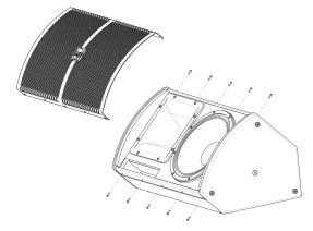
Remove the ESM12 grill, unscrew 10pcs hexagon screws, size 2,5.
