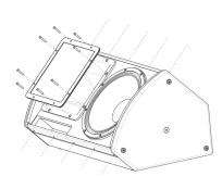
Place the protective cover over the driver horn. Use hexagon screws dismantled from the horn. Tighten the screws.
