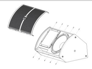
Place the grill and tighten the screws.
