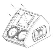
Remove 4pcs hexagon screws, size 2.5 from positions as shown.
