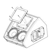
Place the protective cover over the driver horn.
