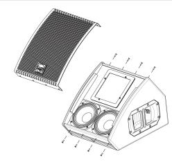
Place the grill and tighten the screws
