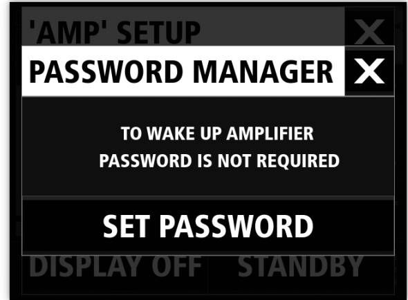
Pic 57: You can SET PASSWORD which will need to be entered to access amplifier when it is in STANDBY mode or if its DISPLAY is OFF. Once set, you can CHANGE the password or DISABLE it.
