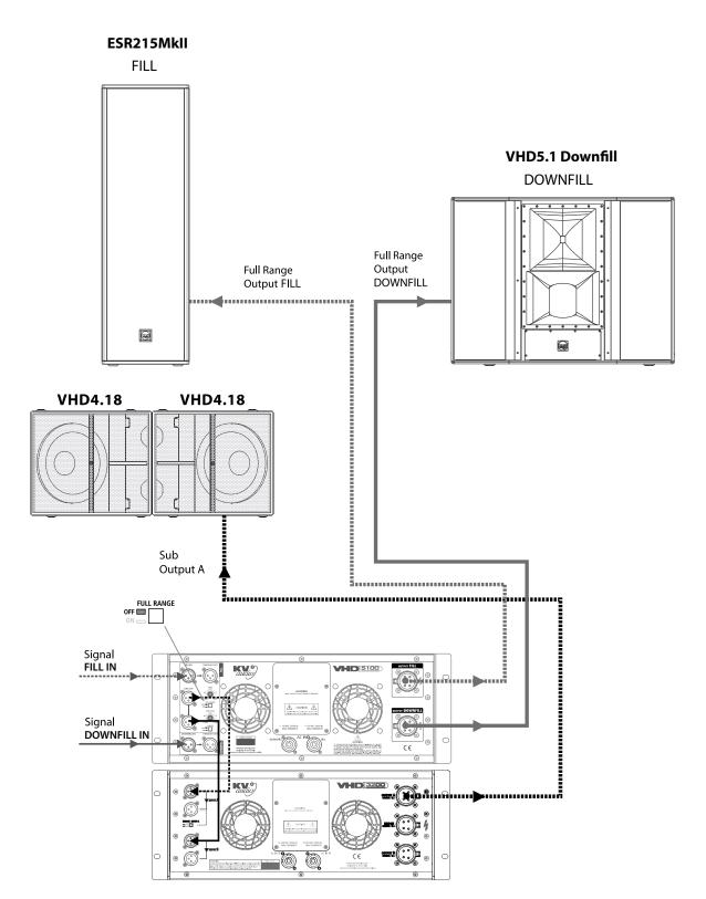
Set VHD5100 Amplifier to FULL RANGE OFF mode. Signal is crossed over at Hi/Mid for ESR215MkII cabinets and SUB for external subwoofer. Crossover frequency is app. 70Hz.
