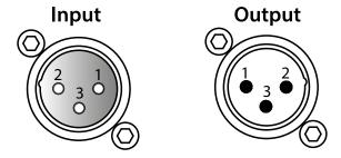
CAUTION: IF IT IS NECESSARY TO CONVERT BALANCED OUTPUT TO UNBALANCED, IT IS IMPOSSIBLE TO SHORT HOT (2) OR COLD (3) PINS WITH GROUND (1). IN THIS EVENT THE LINE DRIVERS WILL CAUSE PERMANENT DISCONNECTION.
