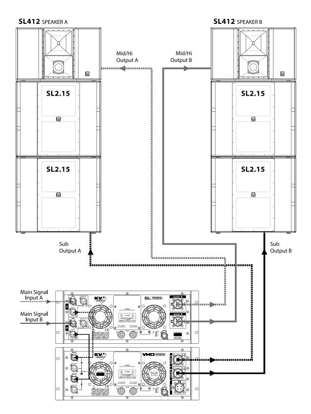
Set SL3000D Amplifier to FULL RANGE OFF mode. Signal is crossed over at Hi/Mid for SL412 cabinets and SUB for external subwoofer.
