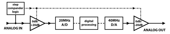
Step compander changes input and output level to increase dynamic range of the converter
