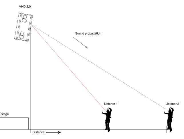
When using one point sound source, the listener in any location gets only a pure (not blurred) sound
