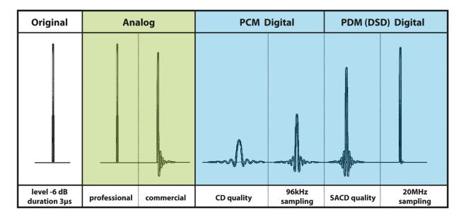
Impulse time response audio systems to input pulse, level -6dB, duration 3µs
