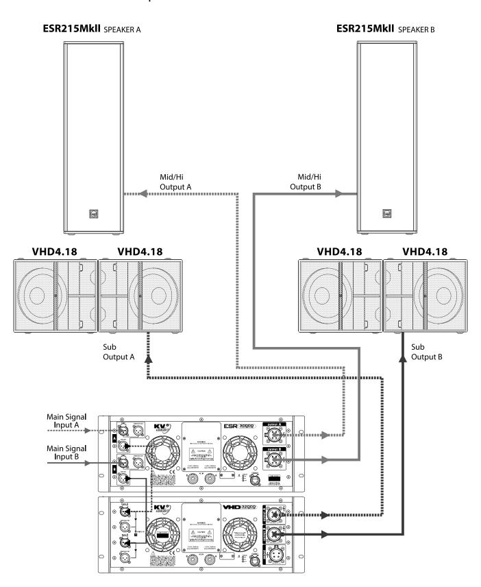
Set ESR3000D Amplifier to FULL RANGE OFF mode. Signal is crossed over at Hi/Mid for ESR215MkII cabinets and SUB for external subwoofer.
