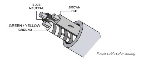
CAUTION: THE ESP1000 REQUIRES A GROUND CONNECTION. ALWAYS USE A GROUNDED OUTLET AND PLUG.
