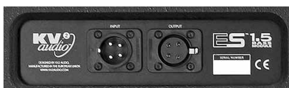
ES1.5 rear panel (cable connection to EPAK unit Amplifier/Controller)
