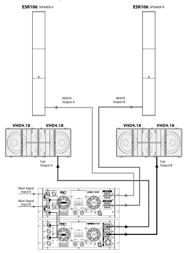
Set ESR2600D Amplifier to FULL RANGE OFF mode. Signal is crossed over at Hi/Mid for ESR106 cabinets and SUB for external subwoofer.
