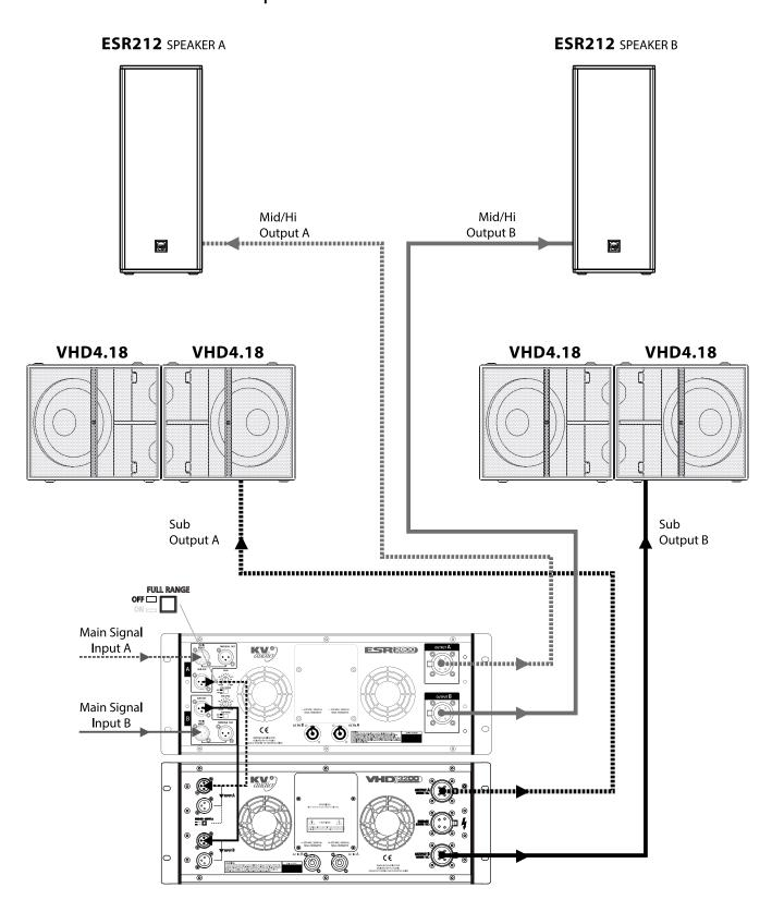
Set ESR2800 Amplifier to FULL RANGE OFF mode. Signal is crossed over at Hi/Mid for ESR212 cabinets and SUB for external subwoofer.
