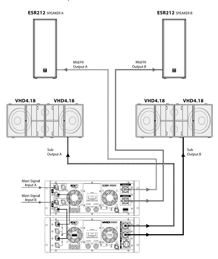
Set ESR2800D Amplifier to FULL RANGE OFF mode. Signal is crossed over at Hi/Mid for ESR212 cabinets and SUB for external subwoofer.
