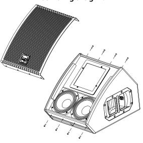
Place the grill and tighten the screws.
