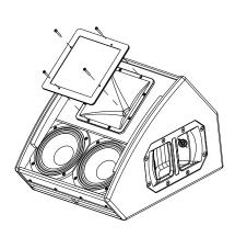
Place the protective cover over the driver horn. Use hexagon screws attached together with the frame. Tighten the screws.
