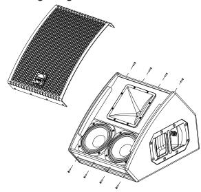
Remove the ESM26 grill, unscrew 8pcs hexagon screws, size 2,5.
