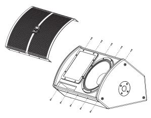
Place the grill and tighten the screws.
