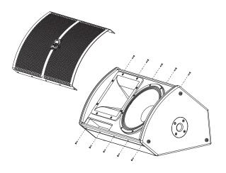
Remove the ESM12 grill, unscrew 10pcs hexagon screws, size 2,5.
