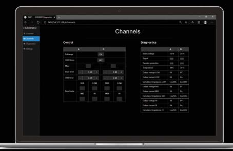
Set up Gain • Operate Mutes • Configure the Limiters • Select Filters, EQ and Bridge modes
